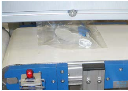
Kits move along the conveyor belt towards the weighing station
